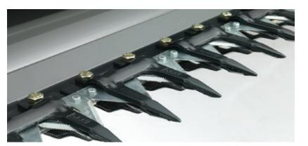
The Schumacher knife is the best performing knife in the business at 1,254 cuts per minute. Self-cleaning and consistently sharp, this keeps the crop moving in tough conditions.
