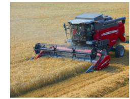
The PowerFlow table improves feeding of all crops and in all conditions for greater productivity. Crops of any height and straw length, from peas and linseed to rye and oilseed rape, are delivered evenly to the main crop elevator for efficient threshing and processing. Bunching and losses are reduced, and the combine can operate at maximum capacity for more of the time achieving higher work rates.
