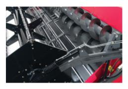
The optional rape auger for the PowerFlow table increases the flow of tall crops into the elevator thereby increasing the output considerably. Two electrical side knives complete the rapeseed kit.
