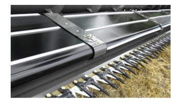
The knife is a massive 1.14 m from the table auger, so vision and performance are optimum. The rugged PowerFlow belts power the crop away from the knife and into the main crop elevator at a consistent speed. The belts also deflect stones rather than taking them into the machine where they might cause damage.
