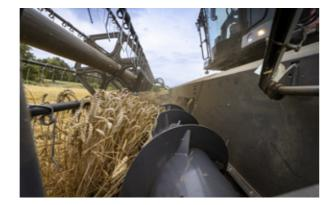
Full width auger fingers on the FreeFlow table increase auger throughput, ensuring positive and fast feed into the main crop elevator.
