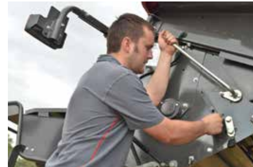
Easy change from chopping to swathing for bales
