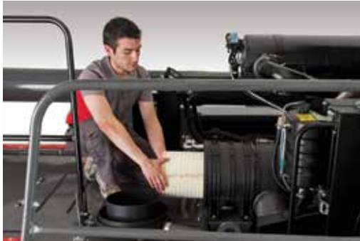
Checking and cleaning the air filter
