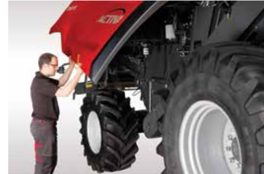
One piece panels with lights allow for quick inspection access with lights for night work
