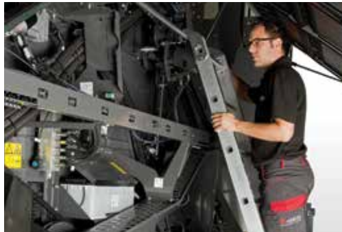
Ladder rail makes inspection easy and safe
