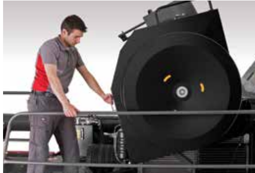
Safe and simple access for radiator cleaning
