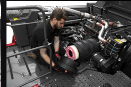
Checking and cleaning the air filter
