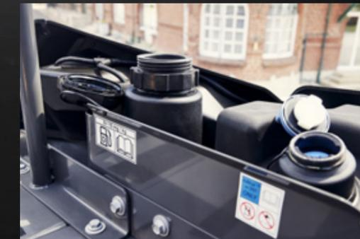
Easy refuelling – the diesel and AdBlue tank fillers are side-by-side for convenient access
