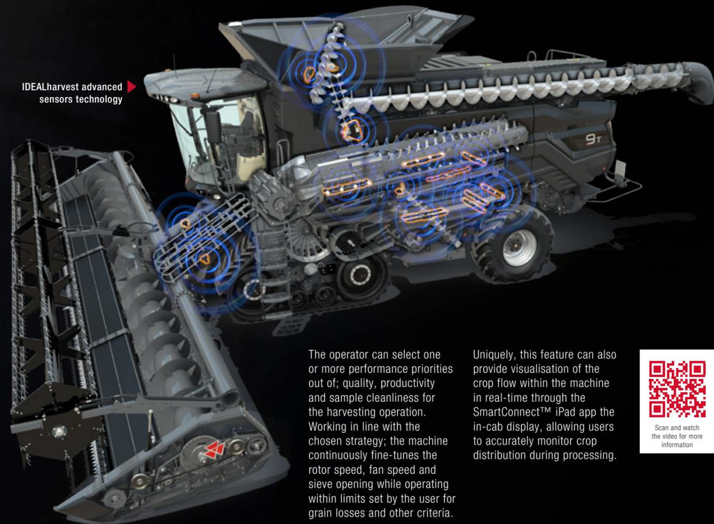
The operator can select one or more performance priorities out of; quality, productivity and sample cleanliness for the harvesting operation. Working in line with the chosen strategy; the machine continuously fine-tunes the rotor speed, fan speed and sieve opening while operating within limits set by the user for grain losses and other criteria.
