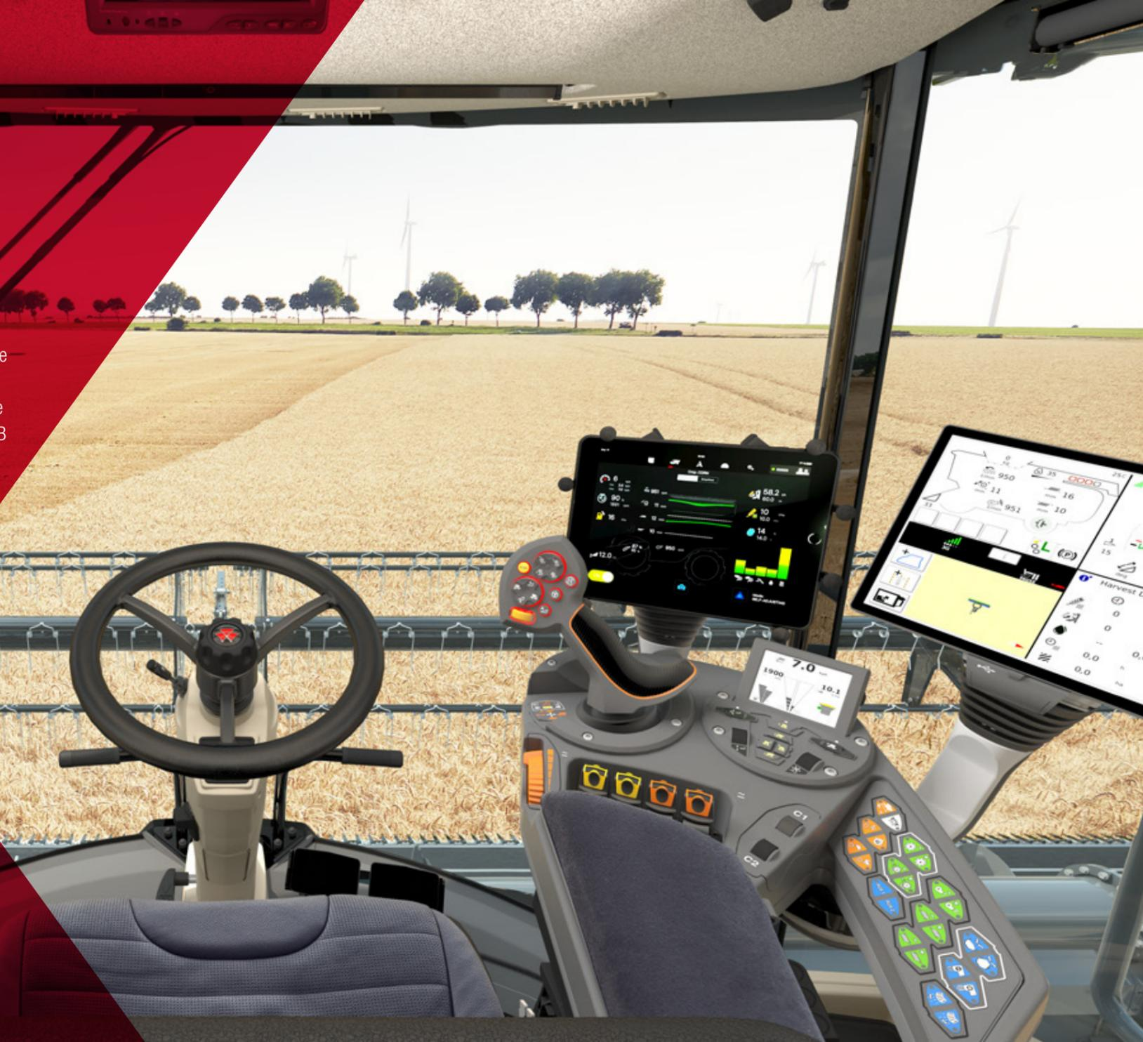
The clear dashboard keeps vital operating data, for example grain losses, in constant view. The ability to move the main TechTouch terminal up to 90° to the operator's right further enhances the view of the header.
