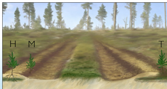
The T21.b creates planting spots with inverted humus (T), mineral soil mounds on inverted humus (H), and mineral soil mounds (M).
