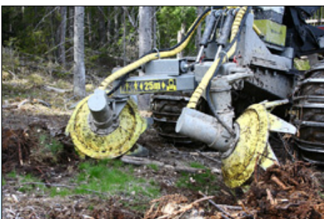
T21.b is mounted on a forwarder of 8 – 11 ton or an agricultural tractor with at least 100 hp
