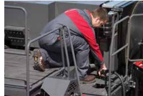
Fuel and AdBlue® fluid access is together for quick attention both have a primary filter in the neck for increased cleanliness.
