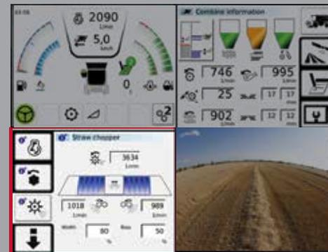
The windows at the bottom of the terminal are called **Info plus screens**. Here the operator can select between various screens giving detailed information on the combine functions. For example the operator sees information at a glance on the engine and shaft speeds and be reassured that all systems are working fine. Yield and moisture information is also seen here .
