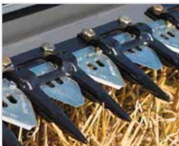
The **Schumacher knife** is the best performing knife in the business at 1220 cuts a minute- self cleaning and stay sharp. This keeps the crop moving in tough conditions.
