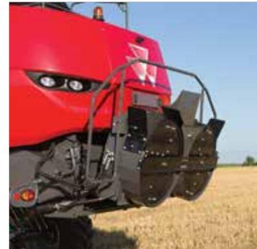
At the **push of a button**, the **MaxiSpreader** can be raised during transportation. This simple procedure takes seconds and no tools are required. The Headland Management system reverses the settings for the MaxiSpreader or the chopper deflectors when turning.
