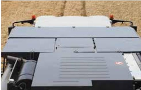
Electrical opening grain tank
