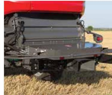
For 9m and 10.7m tables an optional **MaxiSpreader** is available which consists of two rotating impellers which propels the residue evenly over the full width. The speed of these impellers, can be controlled from the cab. If working in windy conditions, the impellers can be adjusted to compensate against any wind force by regulating the speed.
