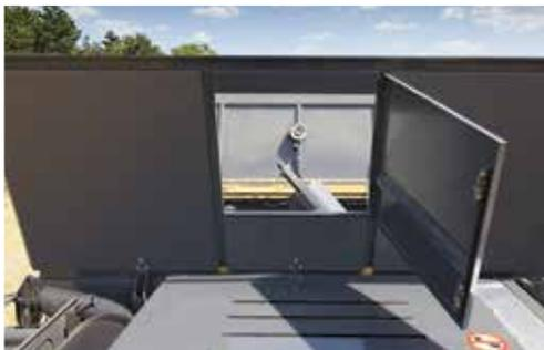
Access is **very easy for cleaning out** or inspection from the engine compartment.
