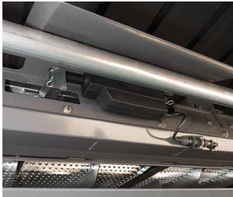
Standard electrically adjustable sieves can be altered from cab but are also part of the one-touch button combine setting system that retains information for future use.
