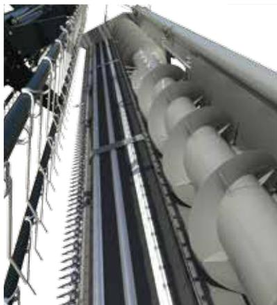
High capacity 762mm **SuperFlow auger** with full width feathering fingers can deliver high speed harvesting in any condition, any crop – no bunching just smooth even feed.
