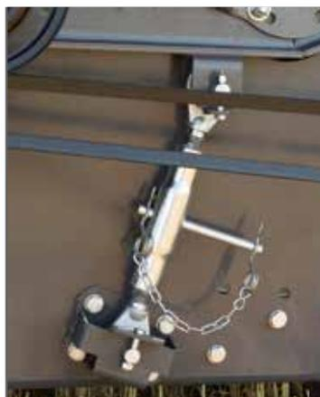
Swift and easy **auger adjustment** encourages operators to change to get the optimum flow for different crops.
