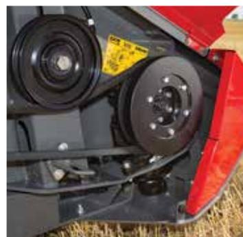
The double drive **Schumacher knife** gives a consistent speed for high output, coupled with far less stress than one drive over 10.7m for added reliability.
