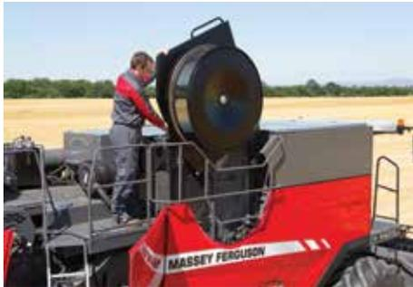
Quick access to cooling radiators for cleaning and inspection reduce downtime and increases fuel efficiency.
