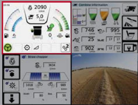
The **General information** screen is always on display in the top left hand side corner of the terminal. It shows engine speed and ground speed. Alongside these are the gauges for fuel, AdBlue®, oil and engine temperature. The graphic also displays the current combine status for the grain tank and the unloader.
