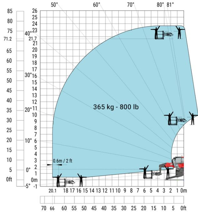
Machine on lowered stabilisers with 1000 kg platform Metric
