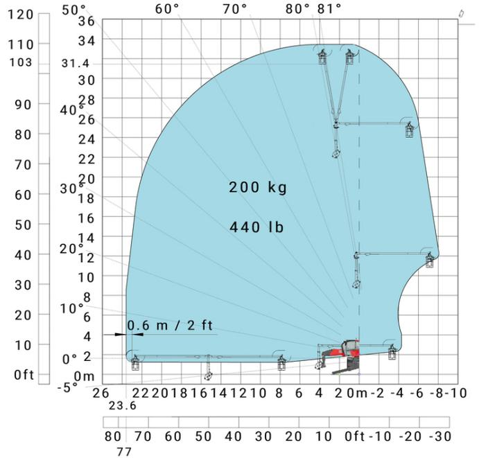
Machine on lowered stabilisers with 3D negative Metric
