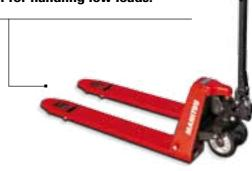
Height of forks in lowered position 51 mm.
